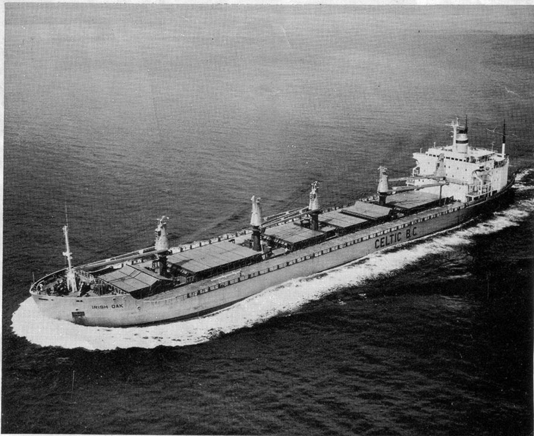
m.v. "Irish Oak", 26,000 tons deadweight; Bulk Carrier; Built: Govan Shipbuilders Ltd., Glasgow, 1973; Port of Registry: Dublin; Service Speed: 15½ knots; Length Overall: 570 feet; Breadth: 84 feet; Class: Lloyds + 100A1.
