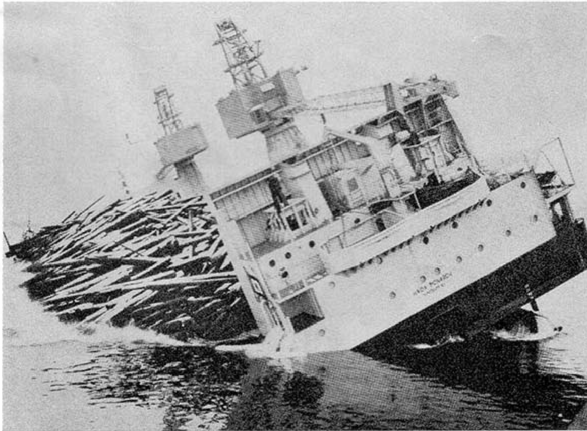
The vessel shown in the accompanying photograph appears to be in difficulties but, happily, appearances in this instance are deceptive. The vessel concerned is the "Haida Monarch", a new self-propelled, self-unloading log carrier which is now in service shipping logs from the Queen Charlotte Islands to Vancouver Island. She is owned by Kingcome Navigation, a Company which has a fleet of tugs and barges operating on the Pacific Coast. On her first voyage the "Haida Monarch", carried 15,000 tons of logs for the firm of MacMillan Bloedel from Gambler Island, in Howe Sound, to the Company's Powell River division
