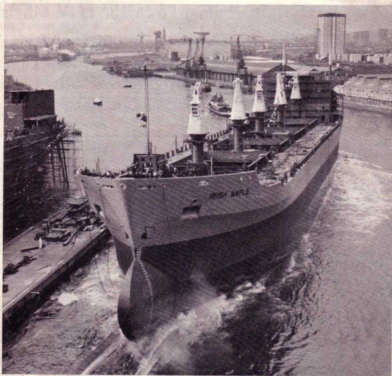
The 26,000 d.w.t. "Irish Maple" going down the slipway at Govan Shipyards, Glasgow on 16th October, the second of four bulk-carriers being built at the yard for Irish Shipping Ltd. The "Irish Pine" was launched earlier this year.
